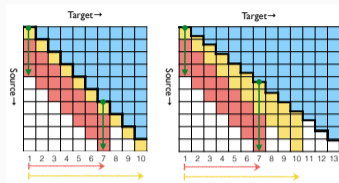
Figure 4: Illustration of our proposed Average Lagging latency metric. The left figure shows a simple case when |x| = |y| while the right figure shows a more general case when |x| \neq |y| . The red policy is wait-4, the yellow is wait-1, and the thick black is a policy whose AL is 0.
